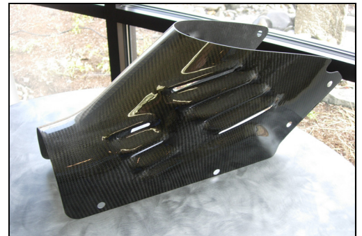
NEW production carbon graphite composite UH-1H 42° gearbox cover
